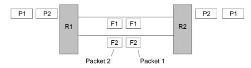
Figure 0-5, Packet transmission with fragmentation, chop-in-half
